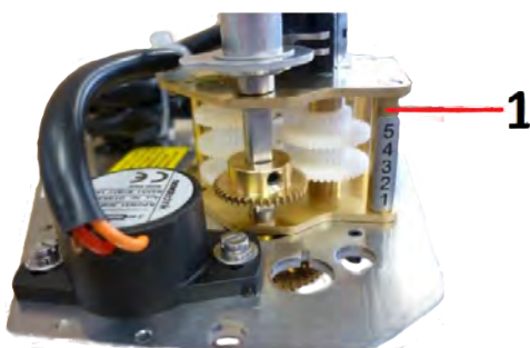
Figure 7.5: Setting the reduction gearing of the limit switching unit for part-turn actuators
