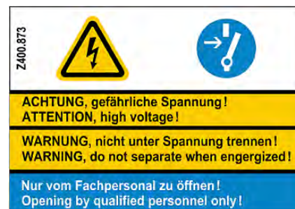
Label with warning of dangerous voltages
