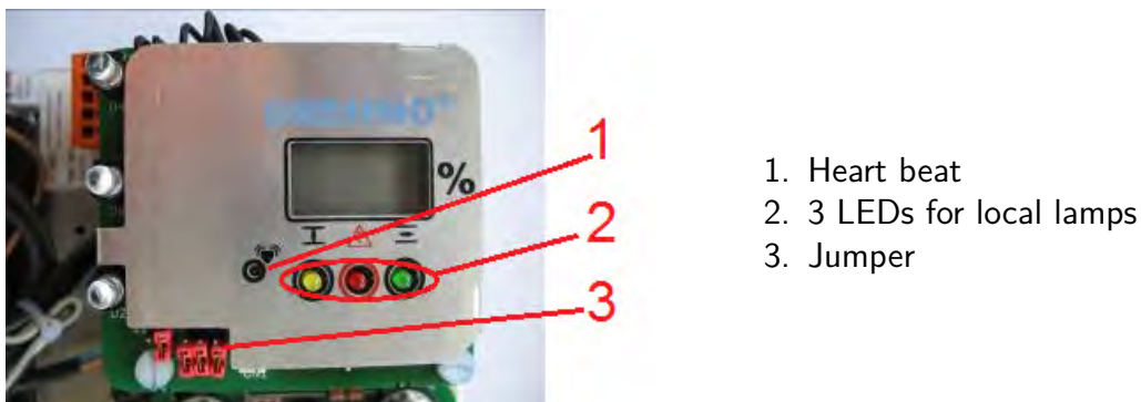
Figure 8.4: LCD-Local control station
